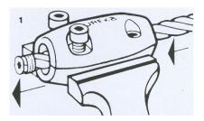
1. Fasten half of the wire rope grip in a vice. Untie the bolts and pull the wire through the lock.
